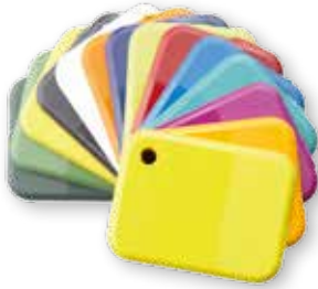
1. Pigmented high-temperature polymers (here PEEK and PES)
