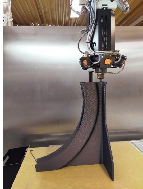
3D printing of the bicycle wheel stand with the Weber additive gantry system (DX) and LUVOCOM 3F PET CF 9780 BK
