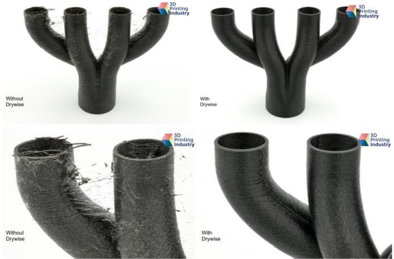
Inlets 3D printed with NylonX non-dried and dried filament. Photos by 3D Printing Industry.
