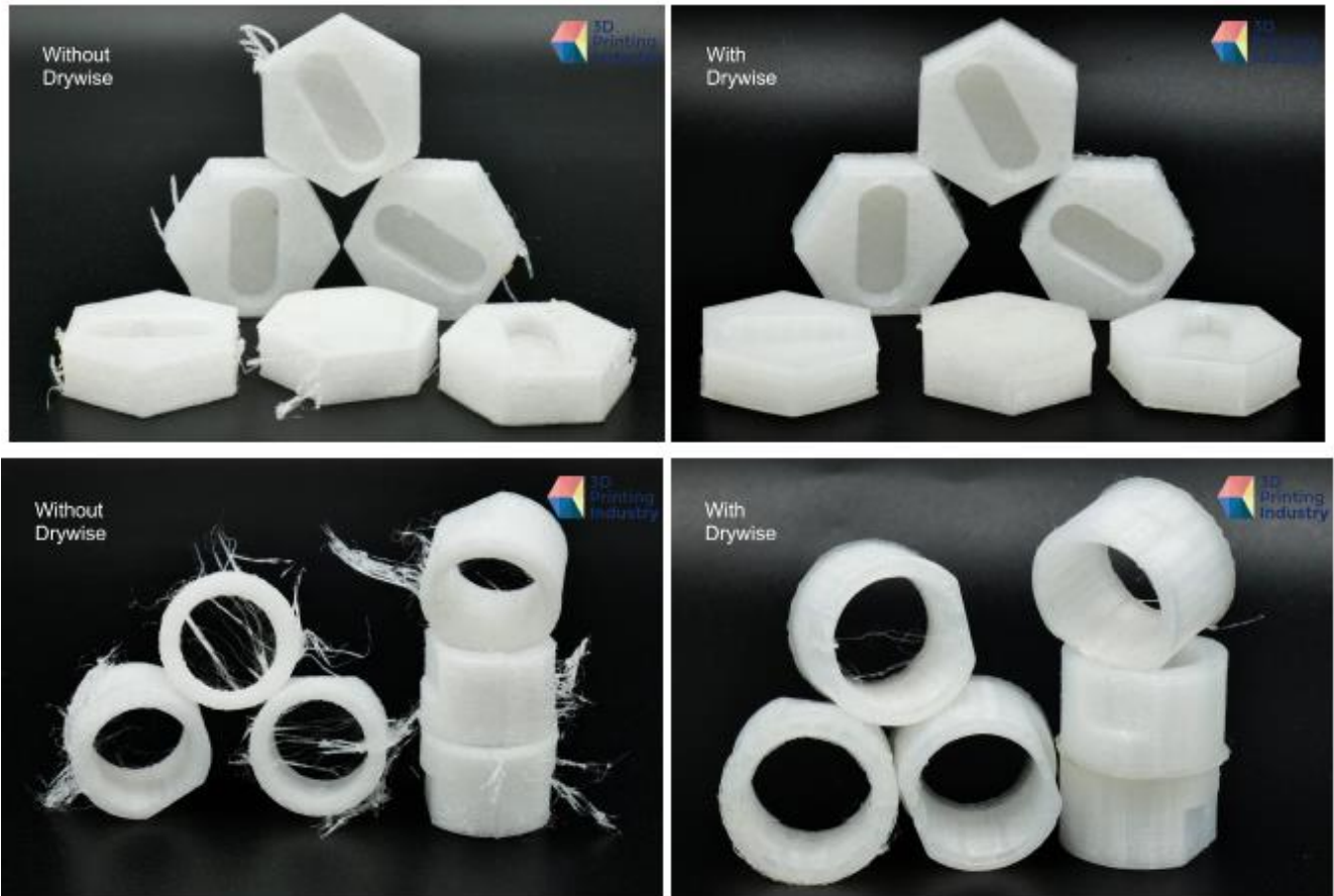
Material hexagon and tube accuracy test parts 3D printed with non-dried and dried BASF PA filament. Photos by 3D Printing Industry.
