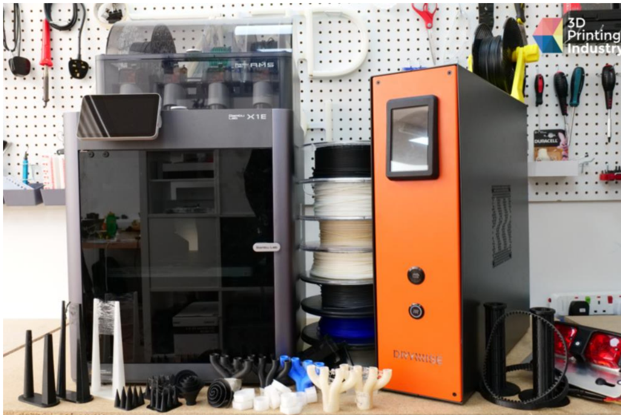
Featured image shows the Drywise filament drying system connected directly to a 3D printer. Photo by 3D Printing Industry.
